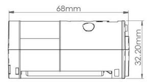
AT2000R module is equipped with infrared sensors at its both ends, which can detect airsoft pellets. User can install AT2000R module into the silencer in any direction according to user's preference and the appearance of silencer.
